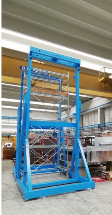
FIG. 3. Picture of the two support structure modules where the detector segments will be mounted.
